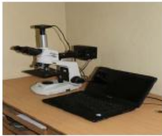
Figure 5. KRUSS metallurgical microscope for measuring tool wears
