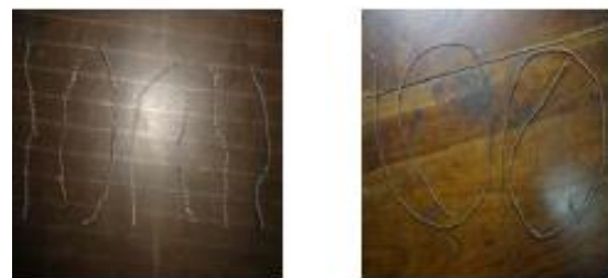
(a) without sound wave (b) with sound wave
