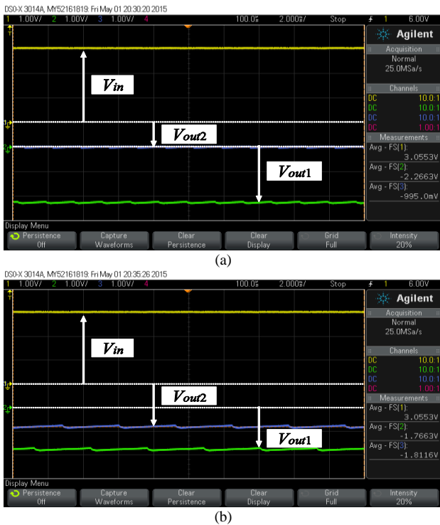
Figure 12. Measured output voltages: (a) traditional control method and (b) proposed control method.
